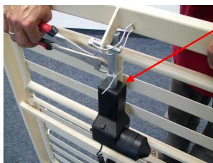
Thigh rest adjustment motor
